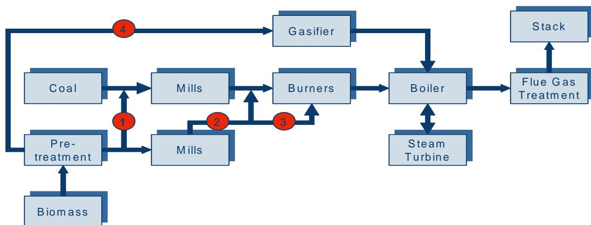
Figure 1. Alternative Co-firing Approaches
