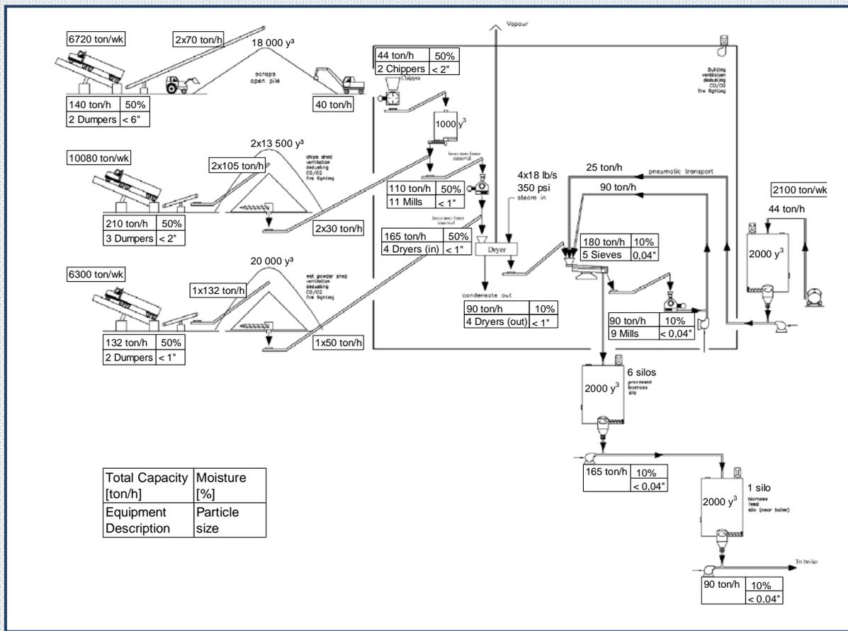
**Figure 3. Layout of Biomass Handling Plant**
